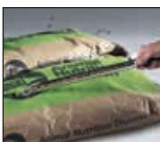
The durable sampler is constructed from chromium-plated brass with light alloy handle and can be sterilized.
